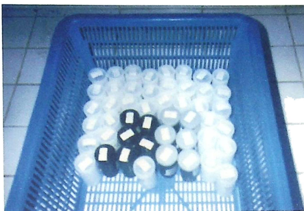
Plate 3. Canisters containing 25 mL acidified treated wastewater samples for Atomic Absorption Spectrophotometry (AAS) analysis
