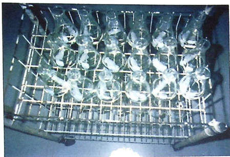
Plate 5. Erlenmeyer flasks containing 100 mL wastewater samples and adsorbents
