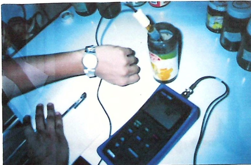
Plate 4: Measurement of redox potential was done in the laboratory.
