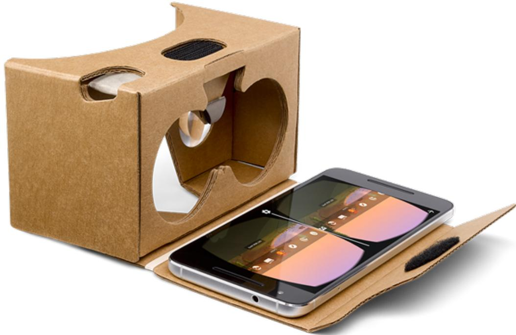
Figure 4: The Google Cardboard with a smartphone displaying a VR application.
