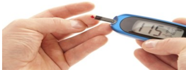
Figure 2: A glucometer device for measuring blood glucose.
