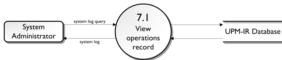
Figure 4.14. Subexplosion of the Process 7.1: View System Log, University of the Philippines Manila – Institutional Repository
