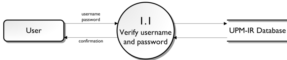
Figure 4.3. Subexplosion of the Process 1: Login, University of the Philippines Manila – Institutional Repository
