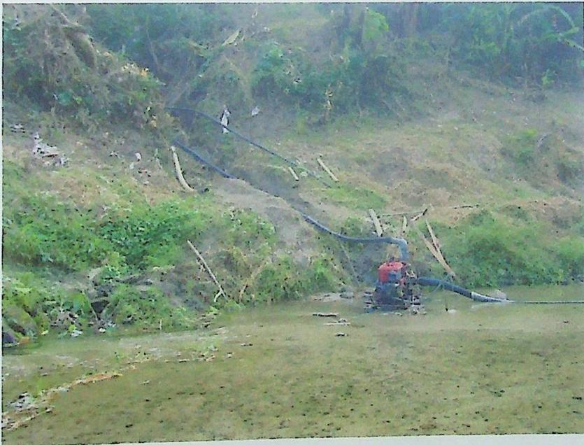
Plate 3. Boundary collection site. Motorized pumps used to pump water to piggeries near the river
