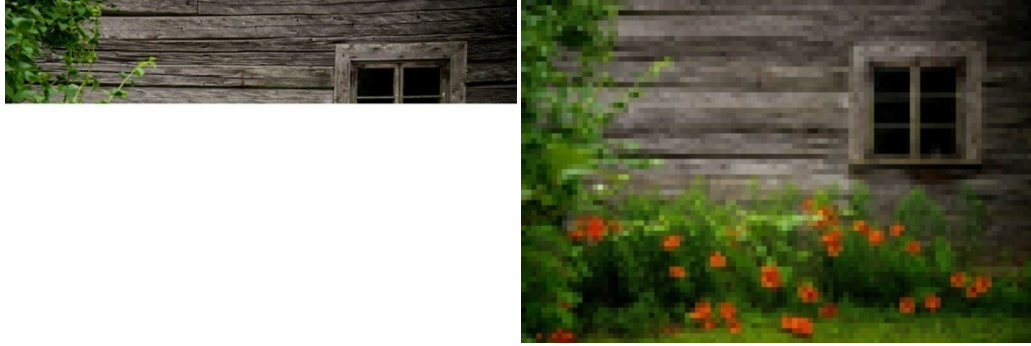
Fig. 7 Sequential JPEG versus Progressive JPEG with 30% of the image loaded
